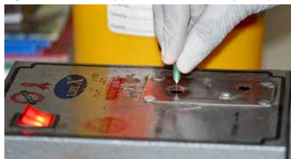
Figure 4 An electrically powered needle destroyer, Nepal
