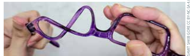
Figure 2 Polycarbonate may snap when twisted.
