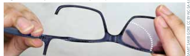
Figure 2 Polycarbonate may snap when twisted.
