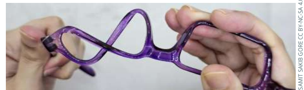
Figure 2 Polycarbonate may snap when twisted.
