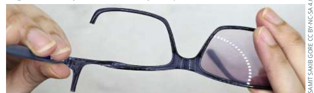
Figure 2 Polycarbonate may snap when twisted.
